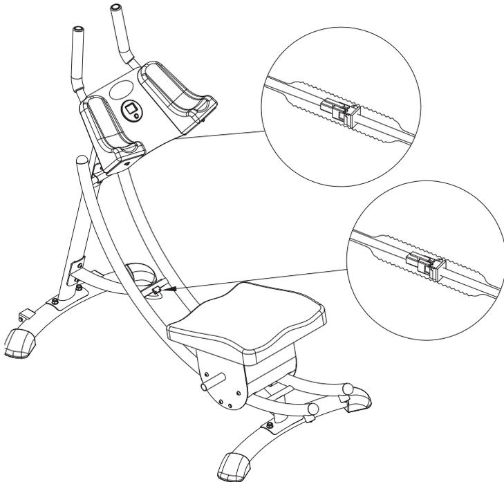
**Step 5:** Connect counter wires in 2 locations as shown. Install wire protection covers to cover wire connections.
