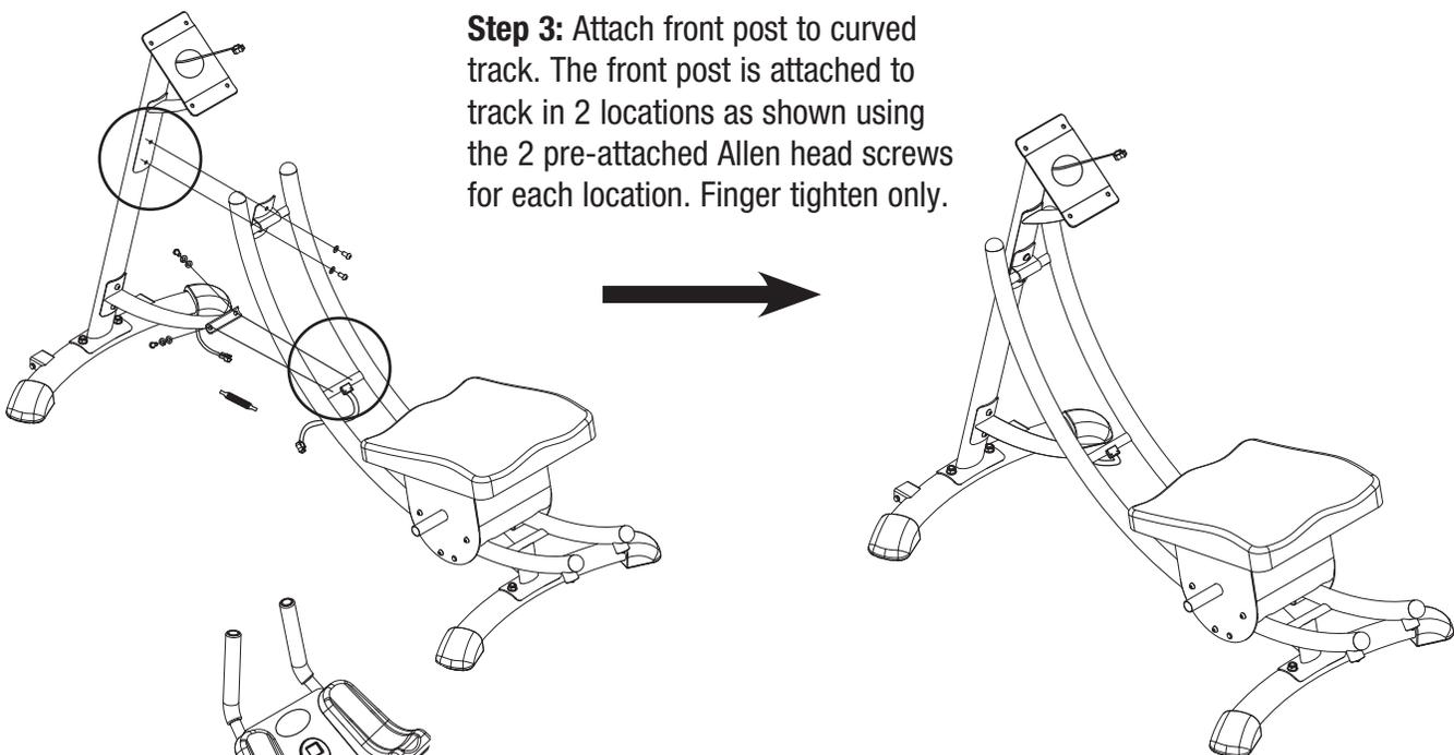
**Step 3:** Attach front post to curved track. The front post is attached to track in 2 locations as shown using the 2 pre-attached Allen head screws for each location. Finger tighten only.
