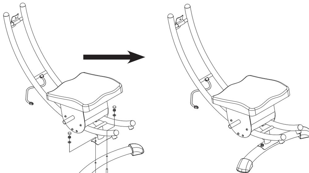
**Step 2:** Attach front foot (with wheels) to front post using the 2 pre-attached bolts. Finger tighten only.
