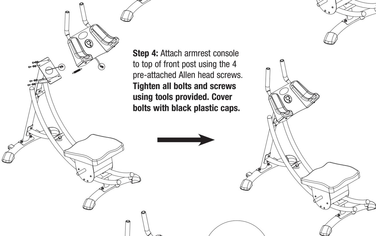
**Step 4:** Attach armrest console to top of front post using the 4 pre-attached Allen head screws. **Tighten all bolts and screws using tools provided. Cover bolts with black plastic caps.**
