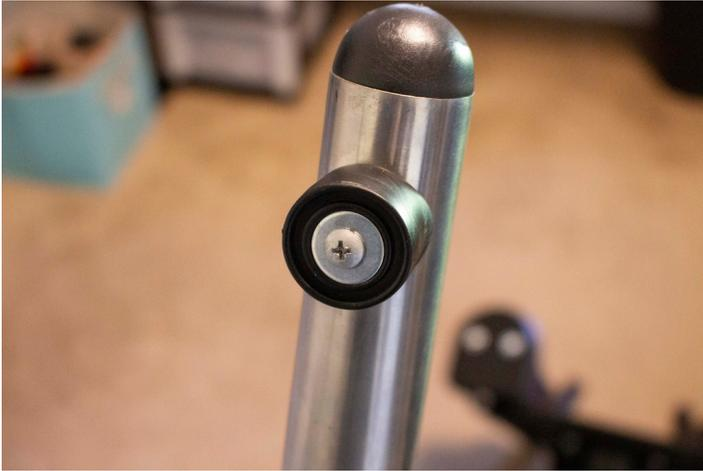
Replacing the home rail bumpers is a very easy task. This will require new bumpers and a Phillips head screwdriver.
