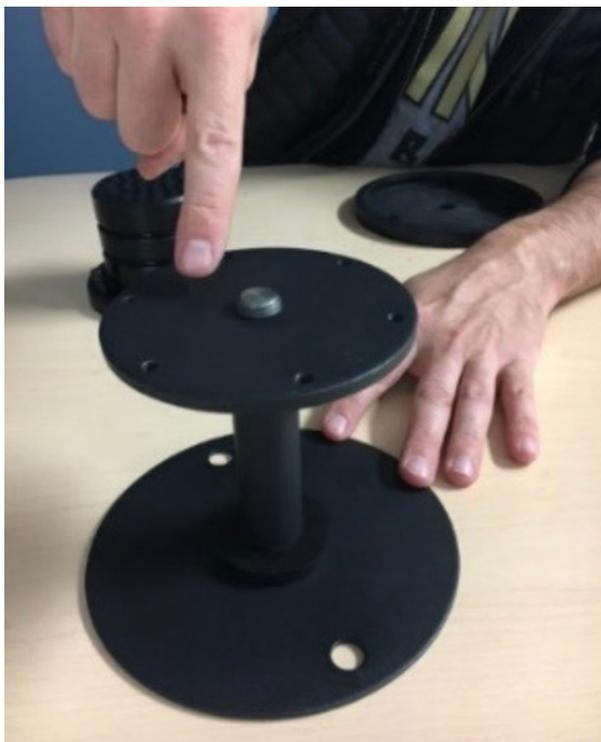
4. Replace top plate with new one. Twist to screw in the new plate.
