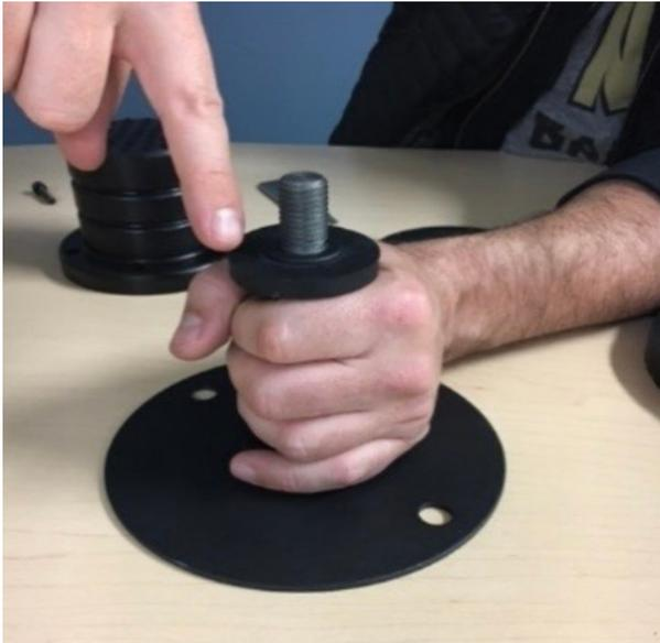
3. Insert new foot through the frame of the TireFlip and put rubber washer on top flat side DOWN. (photo does not show TireFlip frame)
