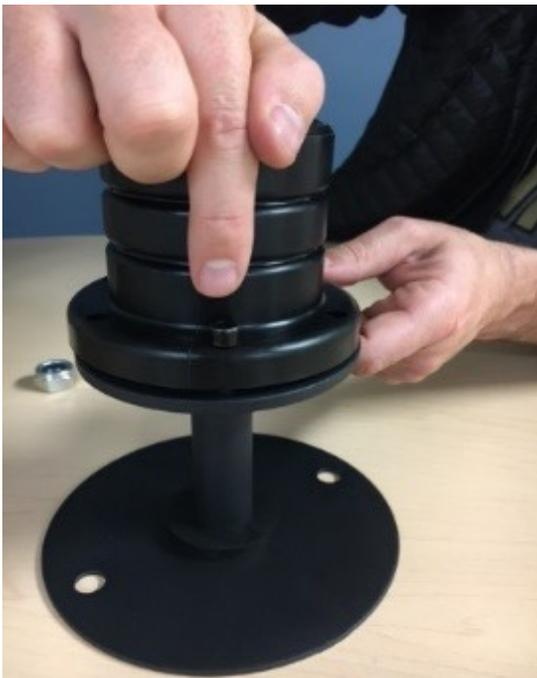
6. Re-attach bumper with M6 bolts using an M6 Metric Allen Wrench.
